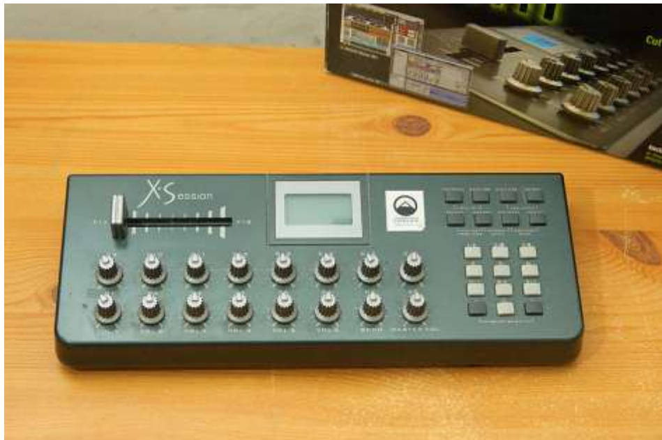
Figure 9. Archetypical MIDI controller called X-Session, basically bunch of potentiometers with not much thought on expressivity. (Moore, 2012)
